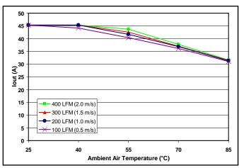
Figure 7: Maximum output power derating curves vs. ambient air temperature for airflow rates of 100 LFM through 400 LFM with air flowing across the converter from pin input to output (nominal input voltage).
