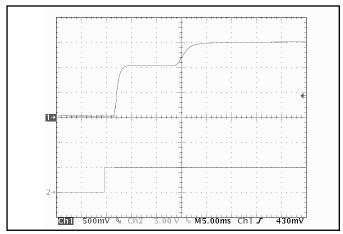
Figure 10: Turn-on transient at zero load (5 ms/div). Load cap:  $10 \mu F$ ,  $100 \text{ m}\Omega$  ESR tantalum capacitor and  $1 \mu F$  ceramic capacitor. Ch 1: Vout (500 mV/div), Ch 2: ON/OFF input (5 V/div).
