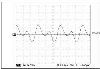
**Figure 14:** Input Terminal Ripple Current, ic, at full rated output current and nominal input voltage with  $10\mu H$  source impedance and  $47\mu F$  electrolytic capacitor (50 mA/div). See Figure 13.
