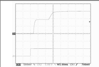
Figure 9: Turn-on transient at full load (resistive load) (5 ms/div). Load cap: 10 uF,  $100 \text{ m}\Omega$  ESR tantalum capacitor and 1 uF ceramic capacitor. Input voltage pre-applied. Ch 1: Vout (500 mV/div), Ch 2: ON/OFF input (5 V/div).
