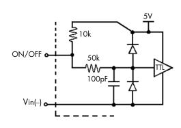
Figure B: Internal ON/OFF pin circuitry
