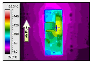
Figure 8: Thermal plot of converter at 35.6 a load current (53.4 W) with 70°C air flowing at the rate of 200 LFM. Air is flowing across the converter from input to output (nominal input voltage).
