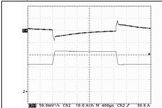
Figure 11: Output voltage response to step-change in load current (50%-75%-50% of lout(max);  $dI/dt = 0.15A/\mu s$ ). Load cap:  $10\mu F$ , 100  $m\Omega$  ESR tantalum cap and  $1\mu F$  ceramic cap. Ch 1: Vout (100mV/div), Ch 2: lout (20A/div).
