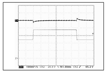
Figure 17: Output voltage response to step-change in input voltage (48V to 75V), at 45A load current. Load cap: 10µF tantalum capacitor and 1uF ceramic cap. Ch 1: Vout (100mV/div), Ch 2: Vin (20V/div).
