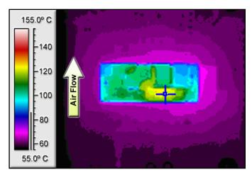
Figure 6: Thermal plot of converter at 36.5 A load current (54.75 W) with 70°C air flowing at the rate of 200 LFM. Air is flowing across the converter from pin 3 to pin 1 (nominal input voltage).
