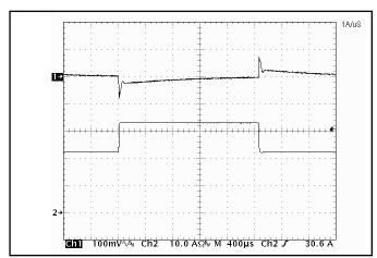
Figure 12: Output voltage response to step-change in load current (50%-75%-50% of lout(max):  $dI/dt = 0.5A/\mu s$ ). Load cap:  $470\mu F$ , 30  $m\Omega$  ESR tantalum cap and  $1\mu F$  ceramic cap. Ch 1: Vout (200mV/div), Ch 2: lout (20A/div).
